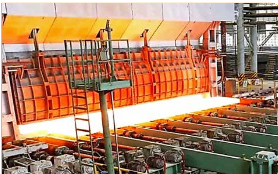
Discharge of a steel slab from a 300t/h walking beam furnace after being uniformly heated using a Flameless Oxyfuel solution with natural gas as fuel, which in future could be partially or fully replaced by hydrogen
